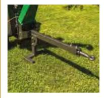
Supporting Feet with Pivoting Drawbar and Towing Eye
