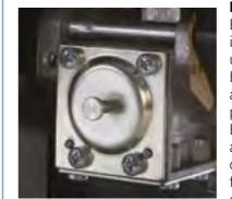
**Enerkit** Each Water Pump is equipped with a unique LPG dedicated ENERKIT carburettor, allowing optimum performance. ENERKIT has an automatic safety shut off valve, stopping the fuel supply when the engine is off.
