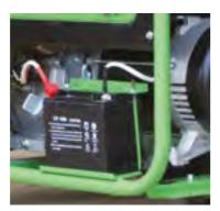
**Battery** The installed onboard battery provides rapid electric ignition and can be easily recharged by connecting it to the appropriate poles on the Generator.
