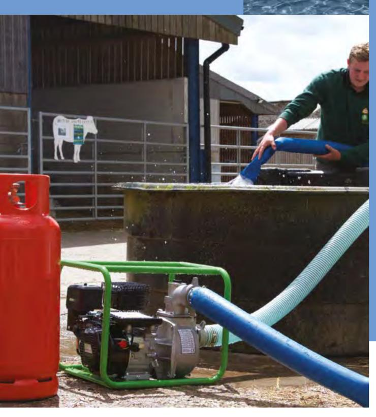
The water pumps are available in 4 different sizes, ranging from clear water to sewage. The pump bodies are ultra-resistant aluminium and are able to move large amounts of water with capacities from 25m3 / h to 70m3 / h. The pumps are ideal for a wide range of scenarios including emptying swimming pools and flooded basements or filling/emptying a water tank. The pumps are ideal for both domestic and commercial users too, including farming and construction sites.
