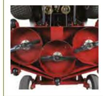
Cutting Deck with Double Blades The double blades allow for flawless precision mowing on a large scale.
